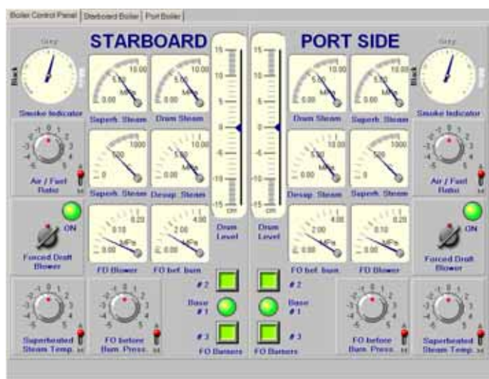
Figure 5: The main boiler control panel.
